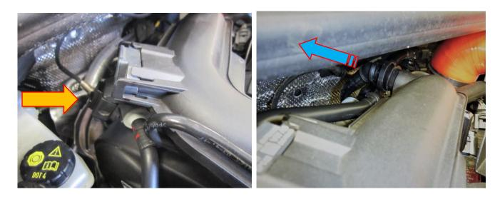
3. Unclip the vacuum hoses and wiring harness from the side of the boost pipe.
