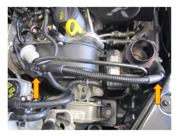
**11.** As pictured below remove the  $2^{nd}$  map sensor from the inlet manifold.
