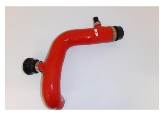
If your vehicle does not have the extra breather fit the machined blanking plug as shown in the picture below.
