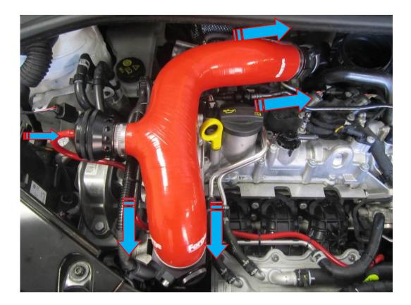
Fit the breather hose to the machined adaptor if your vehicle is so equipped.
