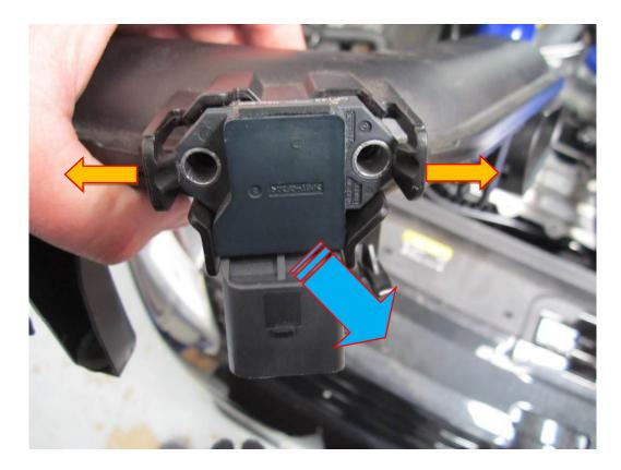
8. Fit the map sensor to the Forge Motorsport billet coupler as shown in the picture below. Use the two M6x12 Allen cap head fasteners provided to secure the map sensor, the blanking plug simply screws into the coupler in a clockwise direction.
