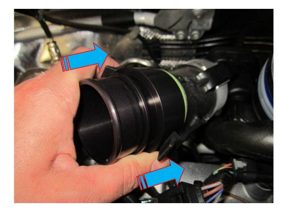
10. Plug in the wiring loom extension between the map sensor and the OEM wiring loom. With the cable ties provided in the kit secure the loom to the OE vacuum pipe, however, leave this until step 13 and secure the loom and the Forge vacuum hose together.
