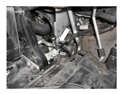
36. Using 2x M8x16mm socket cap bolts and 2x M8 washers secure the expansion tank to the bracket.
