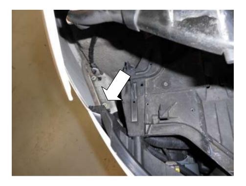
12. Undo X2 T25 Torxs screws on the top of the bumper.
