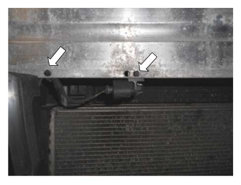
16. At each end of the crash bar unplug both horns and unclip the cable clips.
