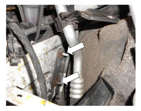
33. Using 3x OEM nuts secure your Forge expansion tank bracket in position.
