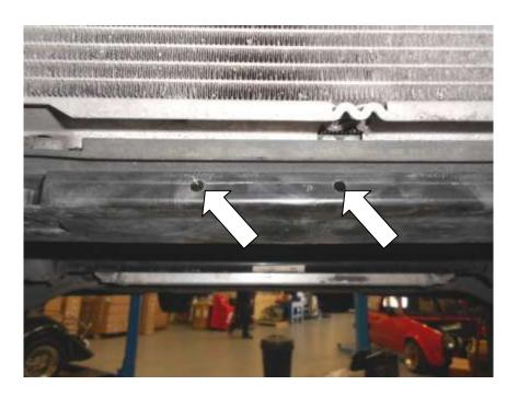
40. Using the 1x T30 Torx screw and M6 washer, bolt the oil cooler in position. Place an M6 Washer underneath the T30 Torx screw.
