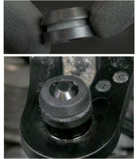
15. Attach the new seal to the original holdfast (of step 9) - these will fit to the hole under the air filter box.
