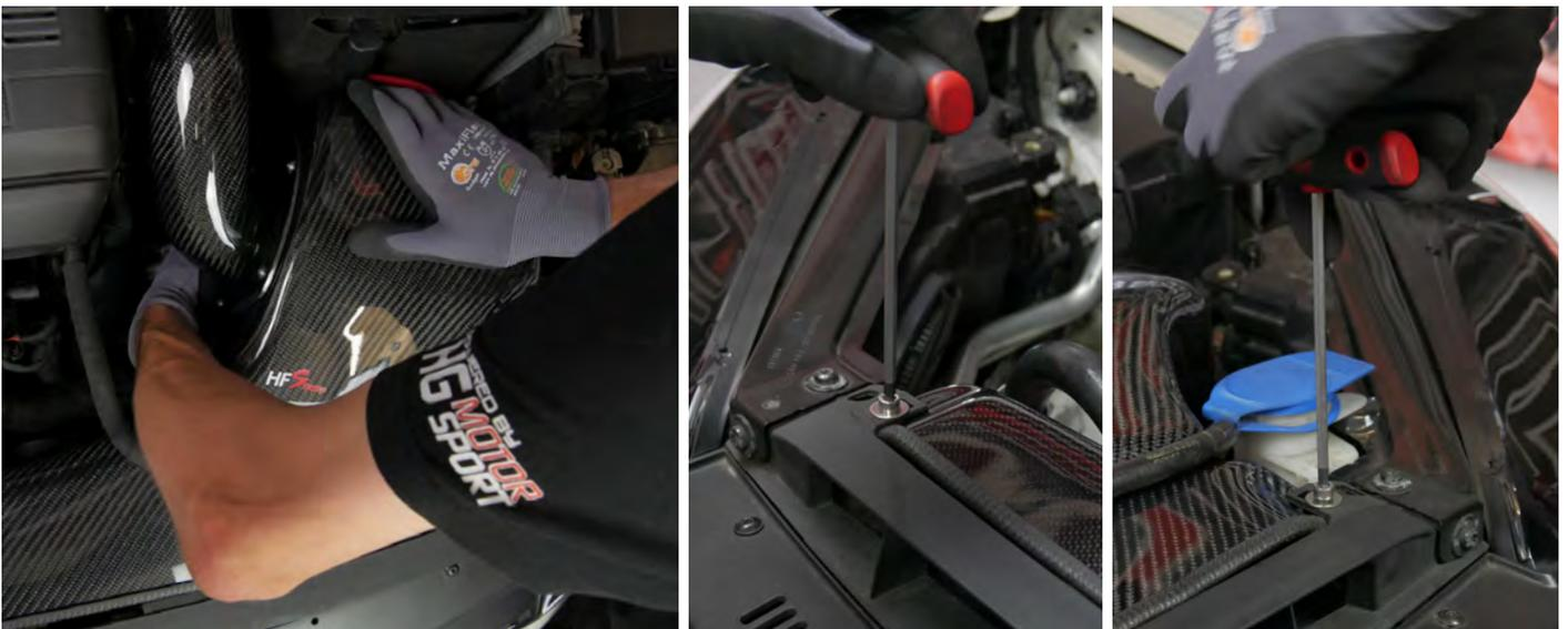
17. Please fasten the intake. For this purpose push the air filter box into the holdfast and bolt on the front of the intake.
