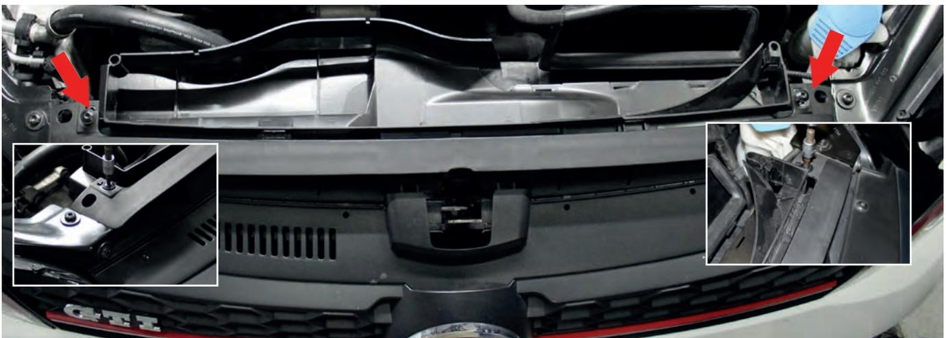
6. Press the left and right retaining clip of the air collector out of the plastic cover of the hood lock support. Then remove the air collector.
