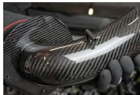
11. To install the vacuum connection, first put in the seal, then press in the bent pipe.
