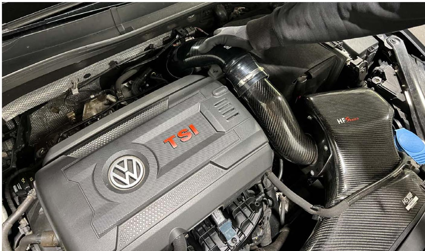
19. Tighten the previously attached clamps.
