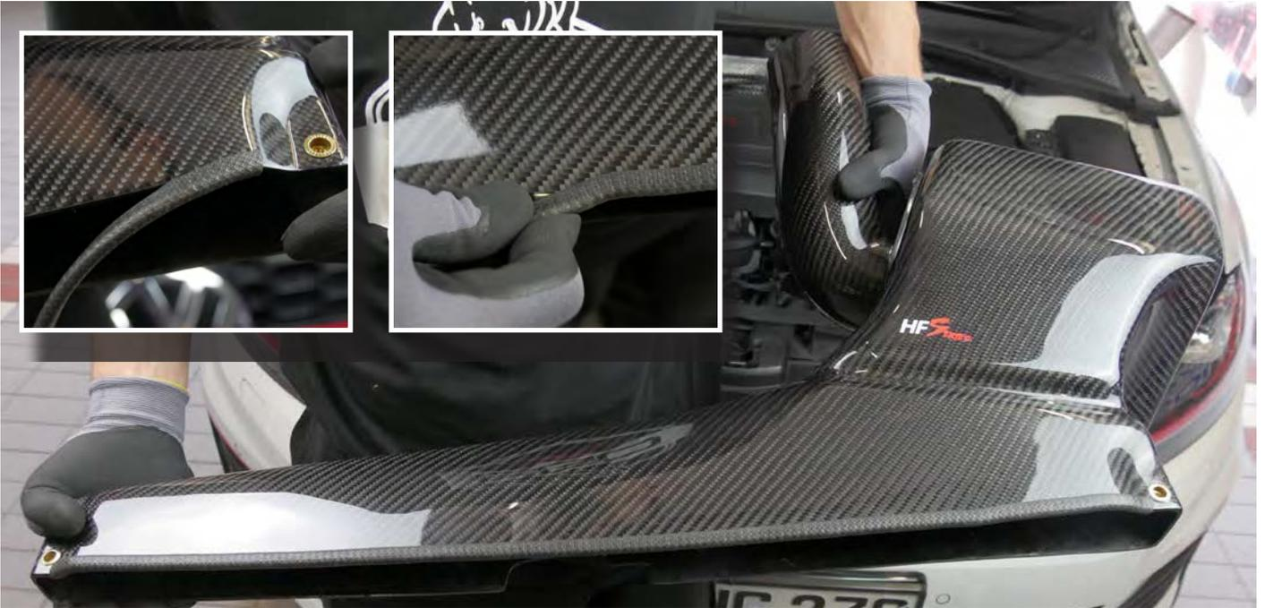
14. Apply the edge protection to the upper edge of the inlet.
