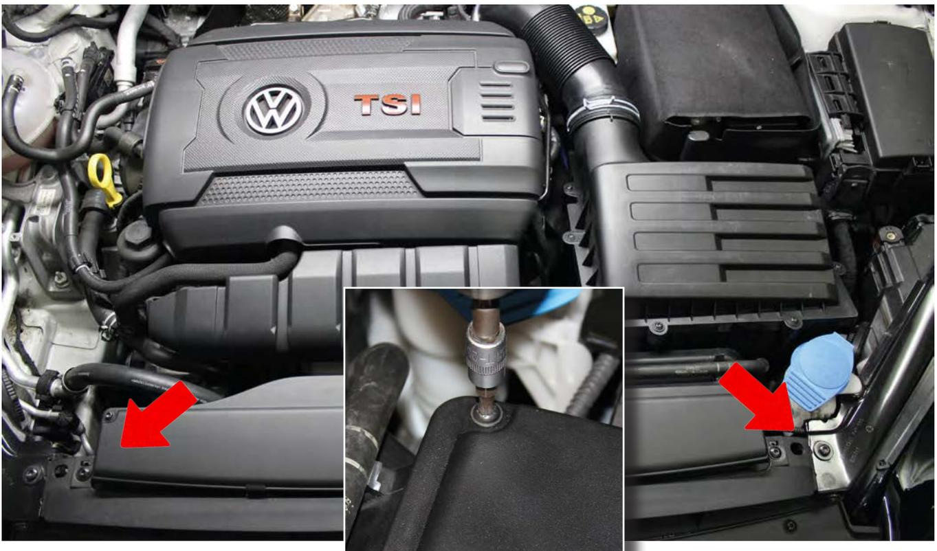
2. Lift the cover of the air collector. Please pay attention on the rear retaining clip and the front retaining lugs. Do not break them.
