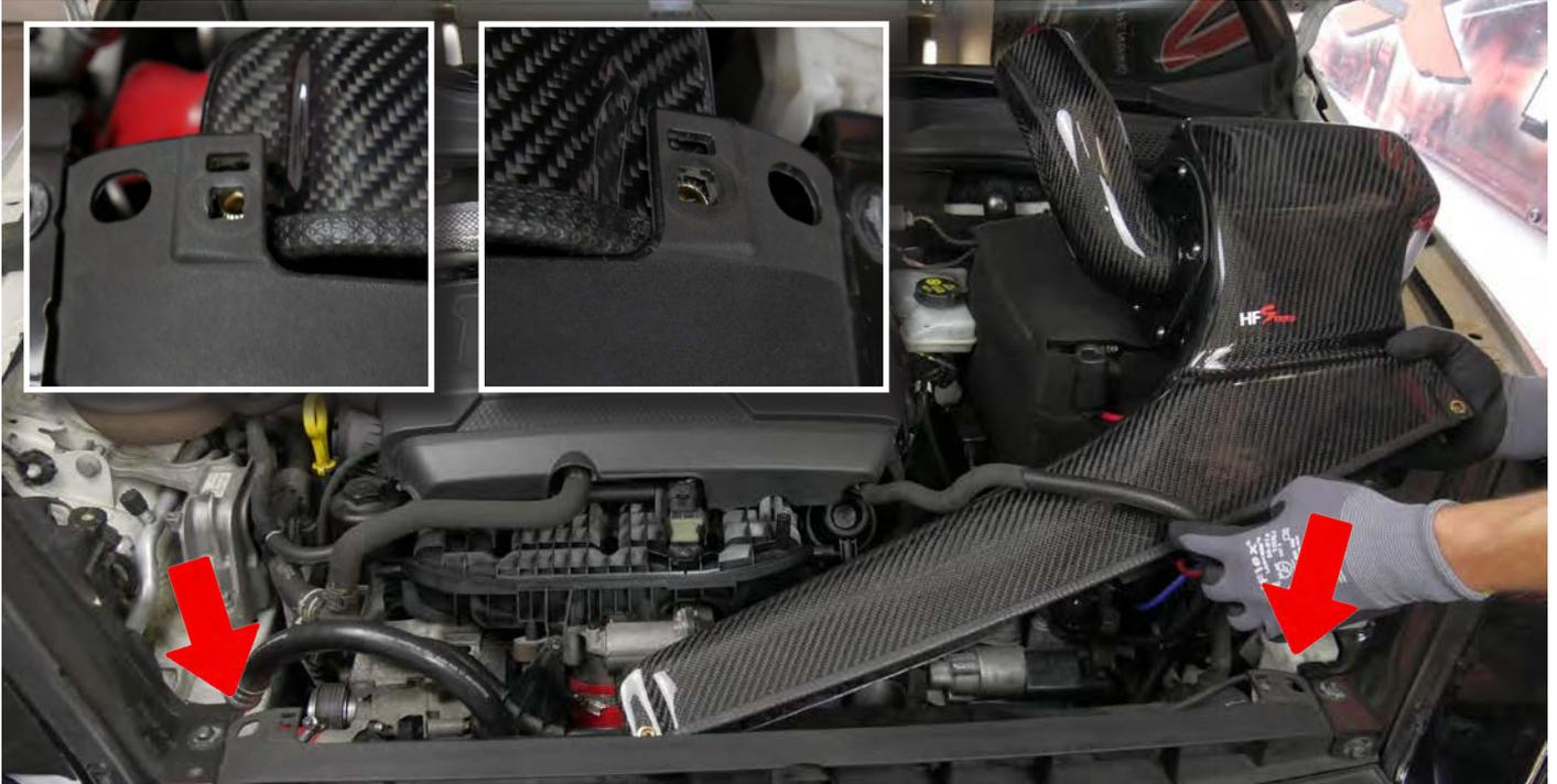
16. Now adjust the complete intake. Pay attention to the two anchorage points in the front. Please connect the vacuum hose to the port on the intake.
