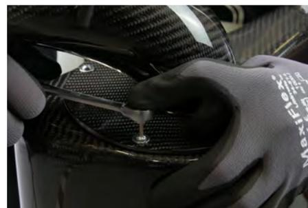
13. Now put in the airfilter and bolt both parts together.
