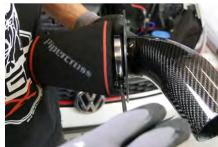
10. Now put together the airfilter and suction pipe and tighten the hose clamp.
