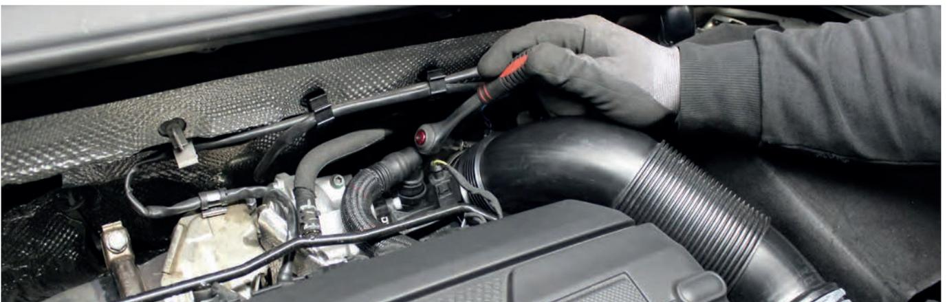
8. Remove the vacuum hose, which is located at the side of the air filter box by simply pulling off the appropriate connection.
