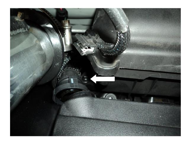
10. Remove the bottom of the air box by pulling upwards to realease it from its rubber mounts, and remove it from the car.
