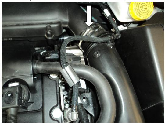
2. Remove the clip holding the breather to the inlet pipe and remove the pipe, remove the moisture sensor wiring and locate to sutible area to avoid the loom earthing on a metal component, and remove the feed to the brake master cylinder by depressing the green push in section and lifting the hose upwards.
