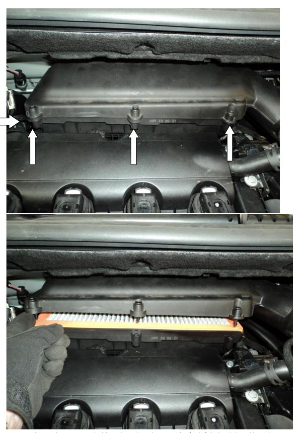
9. Remove the single T25 screw holding the airbox down on the far left behind the oil breather pipe.
