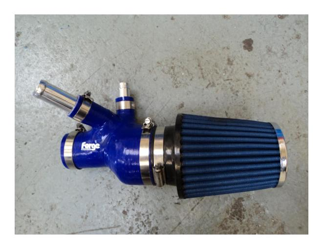
12. Place the intake on the turbo and orientate it so that the pipes on the car line up with the pipes on the intake, then tighten the hose clamp on the turbo, and oil breather lines.
