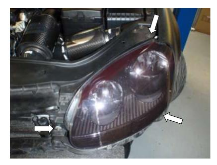
14. Un-clip the fog light wiring that runs along the bottom edge at the front of the car. Also unclip wiring from right-hand side.
