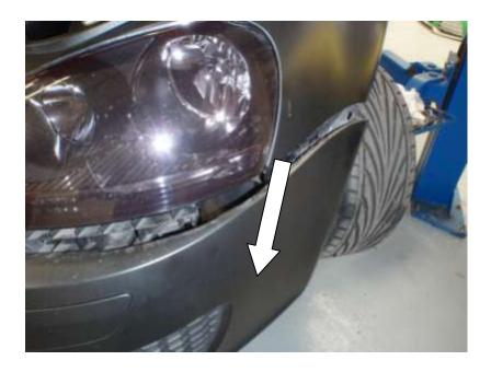
8. This next part requires two people, the first to hold the bumper while the second disconnects the wiring running to both fog lamps.
