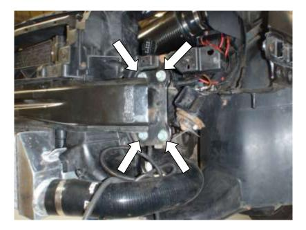
19. Place a trolley jack or suitable support underneath the front clip. This will support the weight of the front end while the final fixings are removed.
