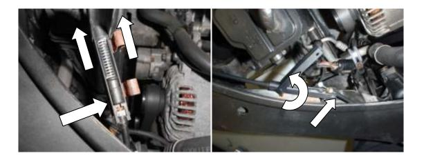
17. Remove 2x T30 Torx screws, to allow A/C radiator/Radiator/Intercooler pack to release from front clip.
