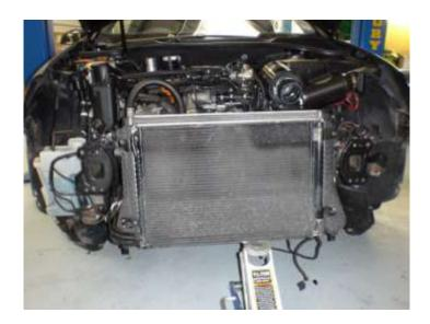
23. Using a flat blade screwdriver remove the sprung clip from the two couplers at each end of the intercooler. Both inlet and outlet tubes can be removed from the intercooler.
