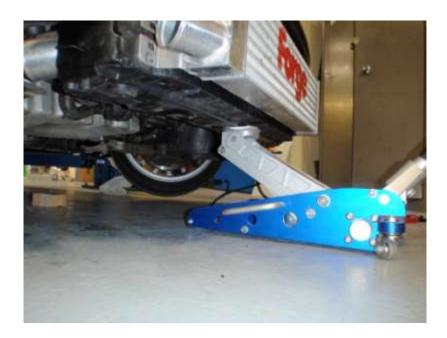
20. While the weight is supported from underneath with the trolley jack, remove the final fixing 2x T30 locate on the top of both wings.
