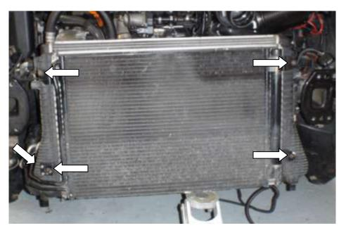
26. Unbolt the A/C pipe work support bracket off the left-hand side of the intercooler.
