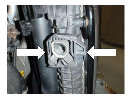
25. To remove the intercooler from the A/C radiator and radiator you will need to support both of them separately. Remove the 4x T25 Torx connecting the A/C radiator to the intercooler.
