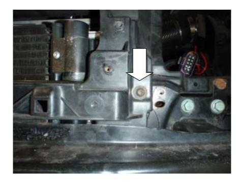
18. Using a 16mm socket remove the 4 bolts located at each end of the crash bar.
