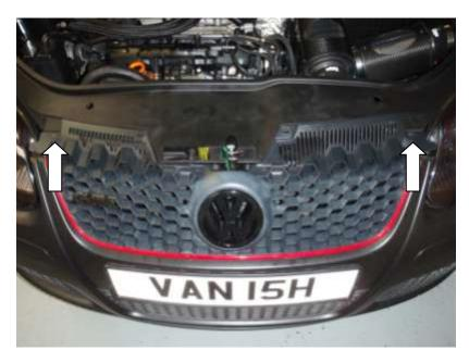
2. Remove the 2x T20 Torx screws form the top of the front grill.
