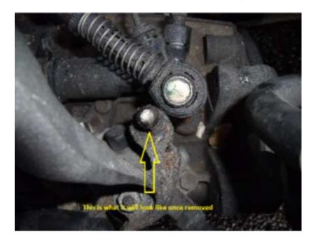
4. Once the ball joint is removed it should look as shown in the picture below.
