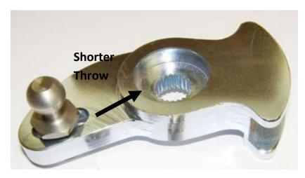
11. Using the grease provided, grease the spine and groove in the shifter.
