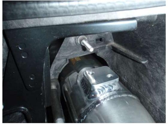
9. Remove the metal bushes from the centre of the rubber grommets supplied, then push the rubber grommets through the holes in the right angled brackets as shown. Once through, push the metal bushes back into position.
