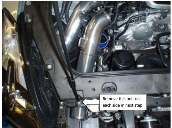
8. Remove the bolt immediately above the pipes on each side (as shown in previous image - on one side it bolts through the bonnet stay), and use the M6x50 bolt supplied, with a penny washer to go through and protrude 30mm the other side, above the pipe.
