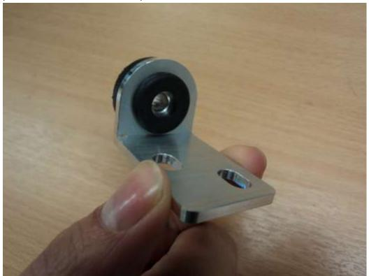
10. Mount the ring spacer supplied over the bolt fitted in step 8, then the right angled bracket, then a penny washer and finally a nyloc nut as shown. Mount the bracket to the tube with the supplied M6 hex head bolts and plain washers. Tighten all bolts and jubilee clips.
