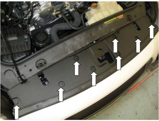
First remove the inlet inside the front cowl – undo the single clip and pull the plastic inlet from the filter (shown with bumper removed, not necessary). Also remove the clip and 10mm bolt holding the air guides in and remove them from the car.
