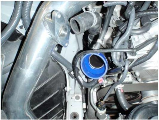
7. Take the pipe shown below and push it through the hole in the cowl first, then rotate it and push down into the silicon coupler. Repeat for the other side.
