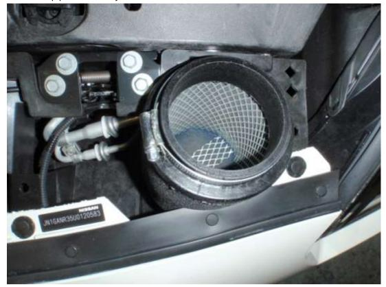
12. Mount the MAF sensors removed in step 3 to the relevant pipes. Tighten with the screws provided and connect the electrical connectors. Replace the dump valves if you removed them, and replace the cover removed in step 1 and the installation is complete. Please now get your car remapped to take advantage of your new found power.
