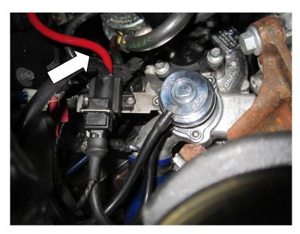
12. Now connect the supplied wiring harness to the Ford connector *(removed in Step 3)* and the solenoid.
