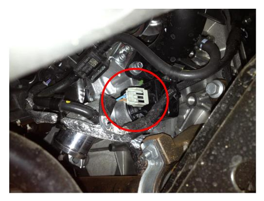
3. Remove the wiring loom from the valve by pushing down on the tab on the rear of the plug .Remove the stock valve from the vehicle by undoing the allen caps with a 5mm Allen key .
