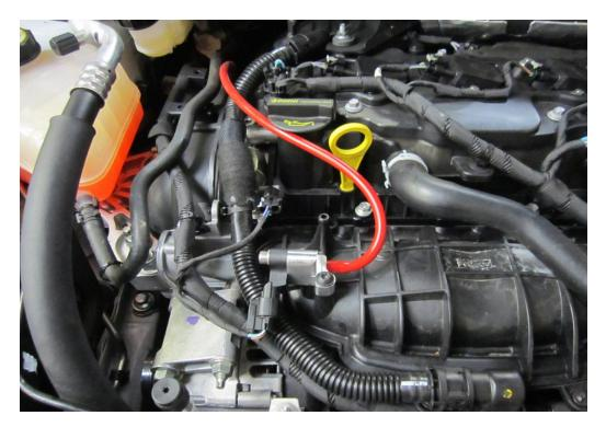
11. The vacuum line that is red (FOR ILLUSTRATION PURPOSES ONLY) needs to be attached to the solenoid. Run this down the back of the engine using the zip locks provided keeping it away from any hot sources or moving parts as pictured.
