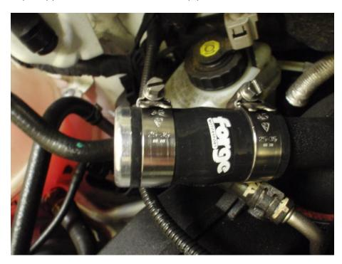
9. Forge motorsport highley recommend venting to atmosphere as this valve has a bigger bore for releasing the boost pressure. However you can install this valve recirculating if you wish. Screw in the small tube supplied in the kit and reattach the stock hose. Follow step one in reverse order and your installation is now complete.
