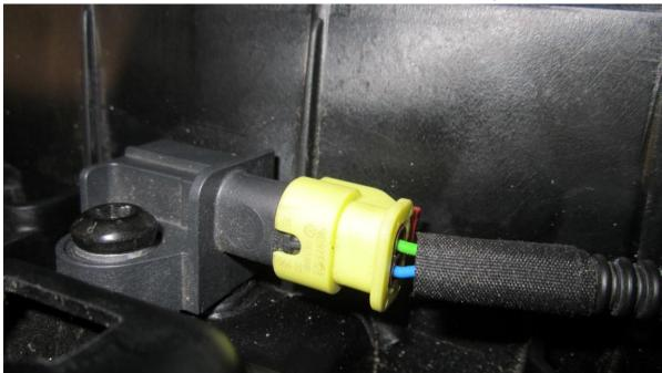
20. Disconnect the loom that's held in place on the lower passenger side of the radiator cowl
