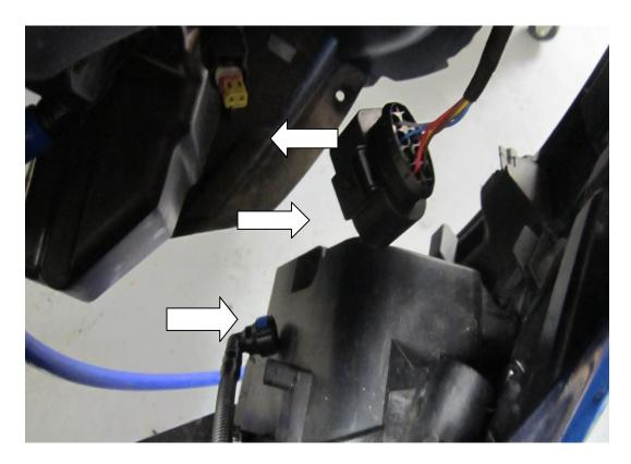
12. Located just behind each headlight are two more T30 fasteners remove both of these .
