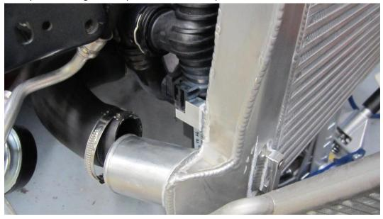
33. Push the clips on your radiator into the brackets on the Forge motorsport intercooler.
