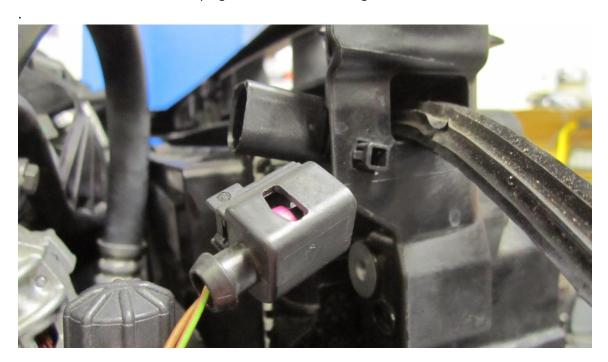
19. Disconnect the loom from the bonnet sensor found in the centre of the plastic radiator cowl
