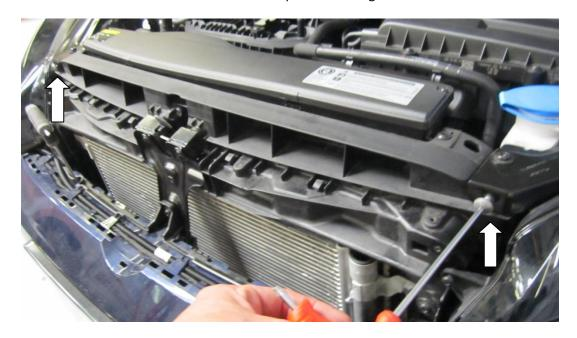
3. Remove the 2x T25 torx fittings holding on the airbox duct .
