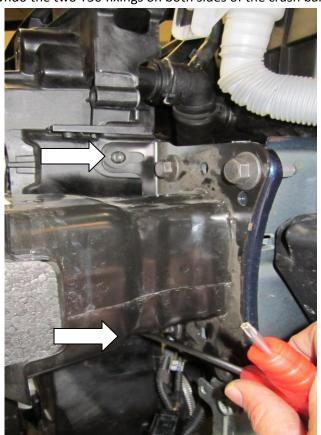
25. Using a 17mm socket and extension undo the four bolts either side of the crash bar holding it place .
