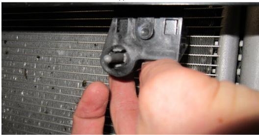
23. Disconnect the plug found also on the radiator cowling.
