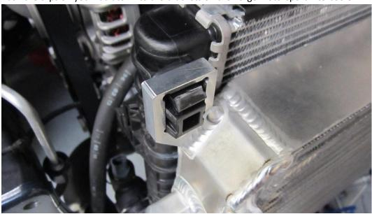
34. Using a 6mm allen key install the clamps on the lower bracket and tighten.
