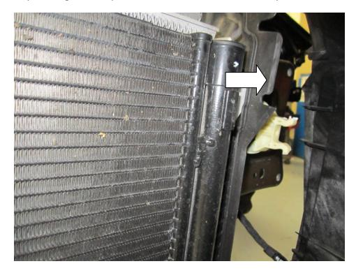
33. Push in the tabs on the top of the intercooler that hold the condensor in place then pulling or pushing the condensor in an upwards motion should remove it from the intercooler. This operation can prove very difficult and is why we recommend having the air con de-gassed.
