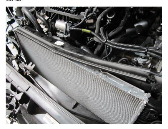
43. Now push the intercooler and radiator into position in the plastic cowling. You may need to use a flat bladed screwdriver to ease the intercooler under the the plastic cowling and into position.
