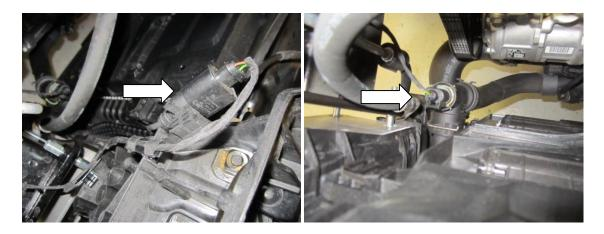
26. Slide the cable box off the plastic cowl, disconnect the bonnet pull, open the top of the cable box and disconnect the grey cable .
