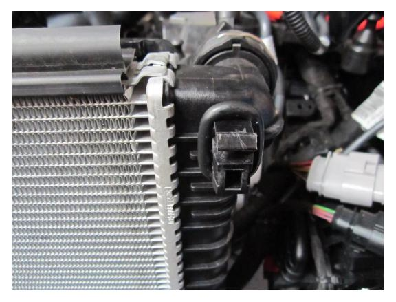
41. Place the radiator into position on the lower mounting blocks, then using a 6mm allen key, tighten into position.
