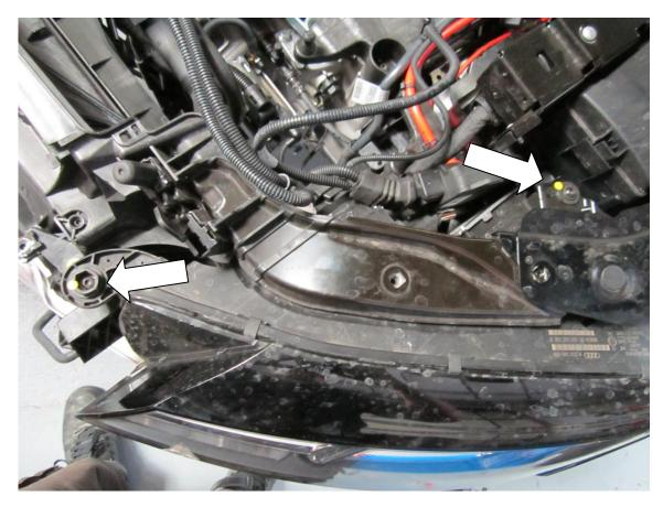
22. Undo the three T30 torx screws underneath the headlight next to the wing.
