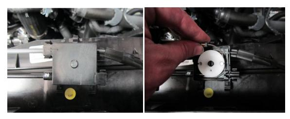
27. Using sharp side cutters cut the tabs from the white blocks that hold the intercooler in place. Dont worry about breaking these as new mounting blocks are supplied with your new Forge motorsport intercooler.
