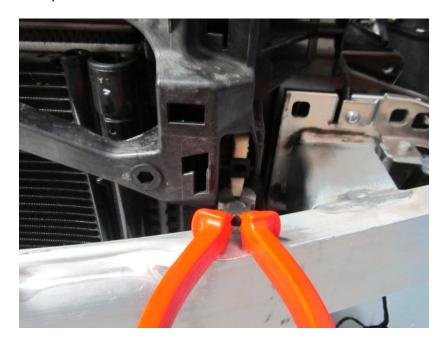
28. We supply longer m8 bolts to help with the install. These will enable you to make sure everything is disconnected and help you to place a jack under the front cowling before removing the crash bar.
