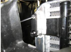
39. Please study the photos below to see where to drill the access holes in order to tighten some of the mounting clamps. The mounting clamp closest to the condensor pipes can only have one of the fasteners tightened dont worry as the cowling itself will hold this in position when fully installed.
