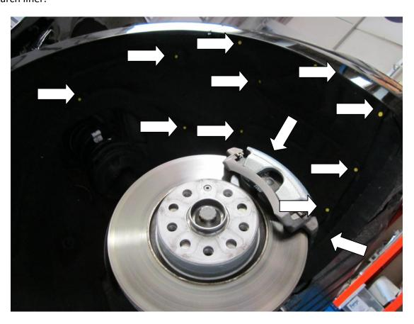
6. Using the T30 Torx drive undo the 3 fasteners pictured .
