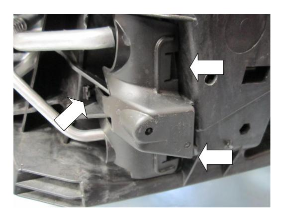
31. Pull the cowling away from you, then using a flat bladed screwdriver push down on the tabs holding the radiator to the intercooler. Push the radiator away from you while the tabs are depressed.
