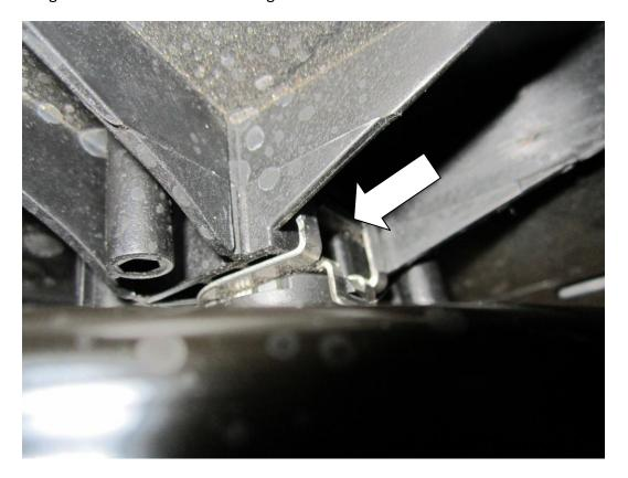
24. The light housing needs to be removed. Pull out the tab that is arrowed in the picture below then slide the housing upwards. Do not undo the bolt under the tab as this will adjust the height of your headlight.
