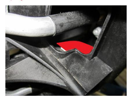
36. Once the front plastic cowl has been trimmed fit the mounting blocks to each side of the intercooler.
