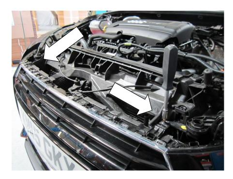
14. Undo the front light washer jet, this can be found behind the front bumper on the passenger side (RHD vehicles).
