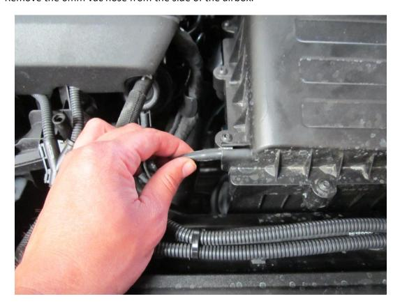
4. Loosen the clamp on the induction hose to your turbo, then pull in an upwards motion to remove.
