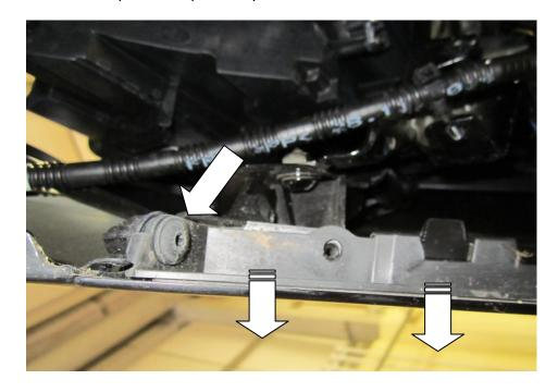
9. Disconnect the wiring loom on the inside the lower passenger side of the bumper (RHD vehicles)
