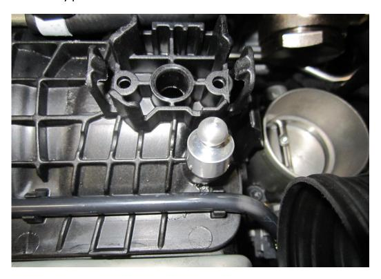
14. The boost source take off adapter must now be fitted to the inlet manifold, place the cork gasket in position first, now fit the adapter by pressing it down on top of the gasket until you feel it click into position.
