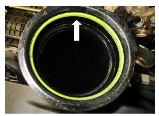
10. Place the o-ring in the groove of the Forge coupler indicated below.
