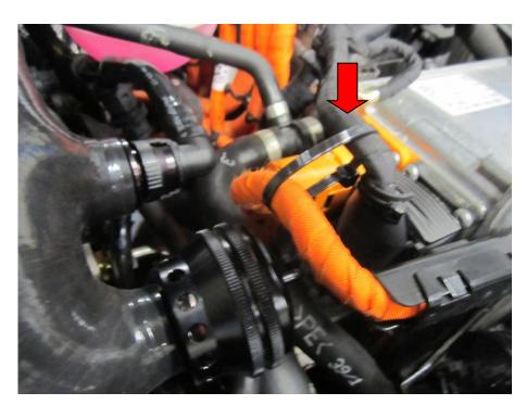
18. Connect the vacuum pipe supplied from the top of the dump valve to the boost take off block you fitted in section 14. Using the cable ties provided, fasten the vacuum tube to the coolant pipe pictured and arrowed white.
