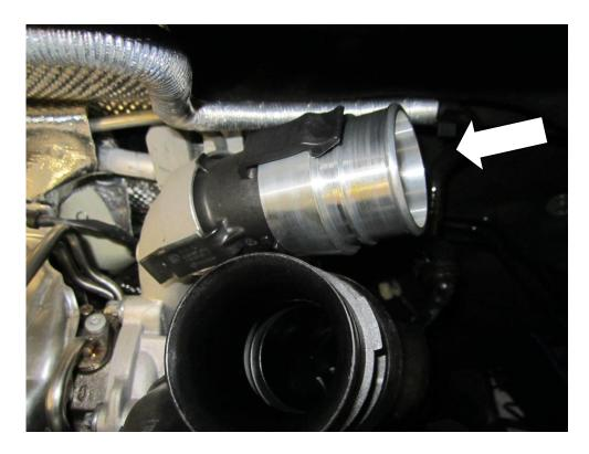
9. Now remove the OEM O-ring from the boost pipe and place it in the Forge throttle body coupler.
