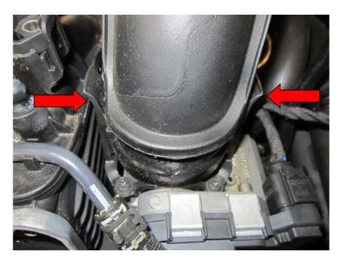
7. Unclip the opposite end of the boost pipe by again prying open the tabs arrowed red, then remove the boost pipe.
