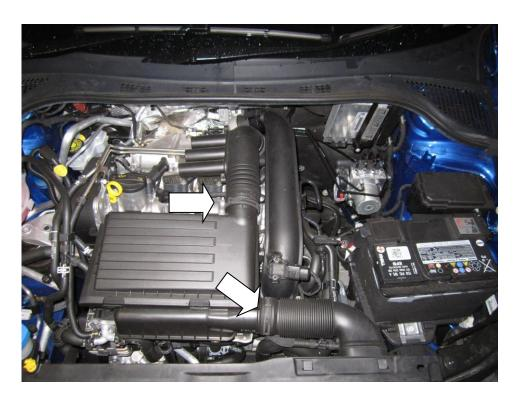
2. Now remove the inlet hose from the slam panel by pushing down on the retaining clips as pictured below.
