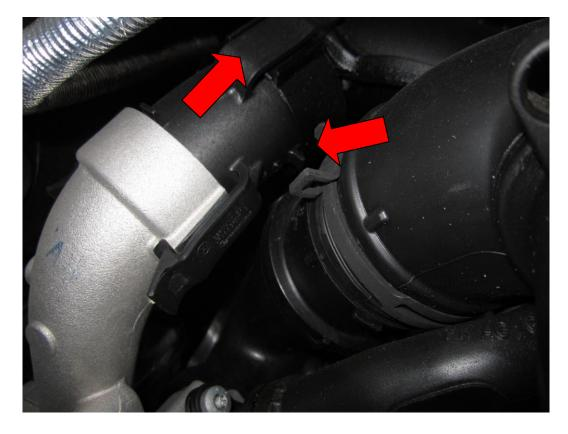
8. Insert the Forge coupler into position by pushing until you hear it click.
