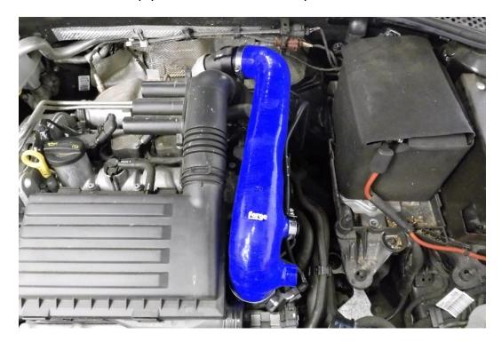
17. Fit the new Forge Motorsport dump valve into the hose and tighten the hose clamp that holds it in position ensuring the cable tie is fitted to the elactric cable to ensure it does not make contact with the valve as arrowed below.
