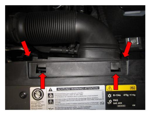
3. Remove the pipe from the airbox to the cam cover breather.
