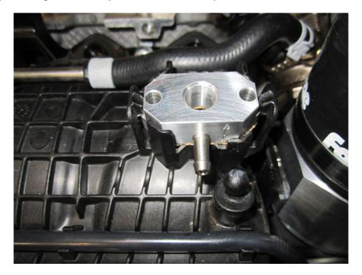
15. Now fit the sensor on top of the adapter using the posi screws provided and tighten with a posi drive screwdriver.
