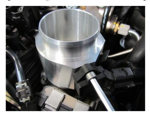
12. Remove the MAP sensor that is mounted on the inlet manifold. Again pry the clips apart while pulling on the sensor.
