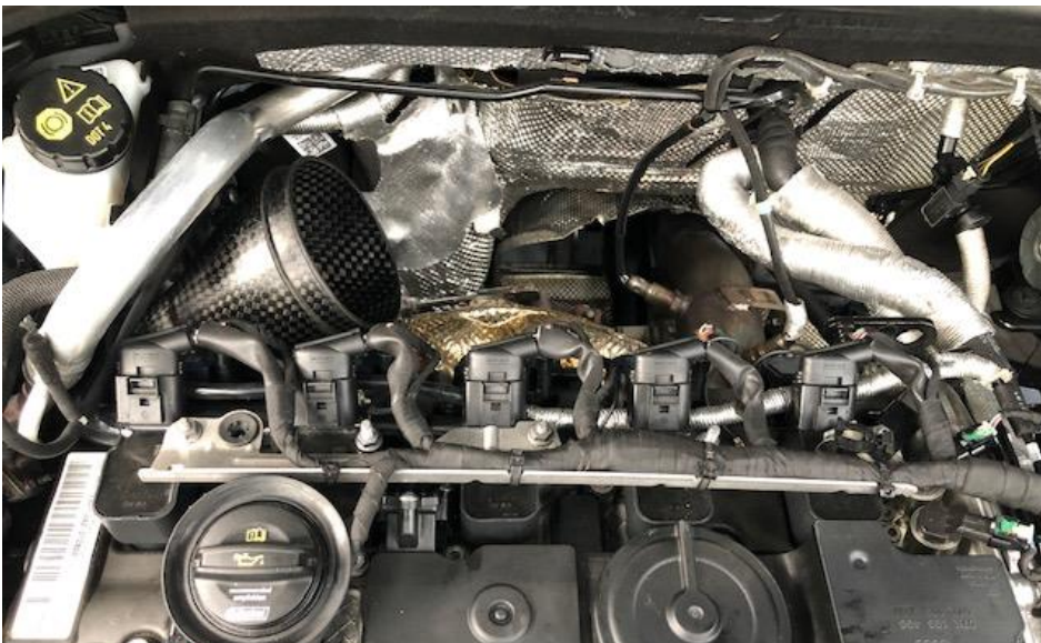
31. Install the coil pack removed previously as well as the loom harness and plugs. Re-attach the undertray.
