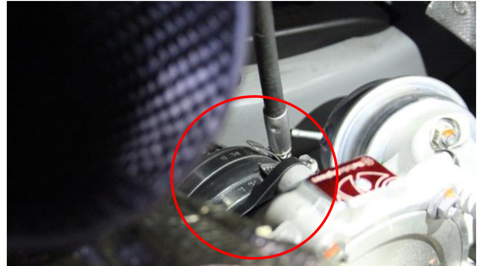
26. Ensure the Carbon tube is still fully engaged in the lower silicon coupler and tighten the hose clamp around the lower silicon. Do not over tighten this with a ratchet. It only needs to be finger tight as the silicon provides a good seal.
