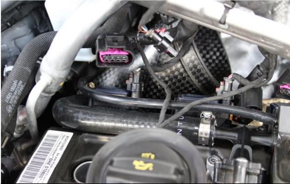
29. Route the vacuum line as shown and behind the carbon inlet tube.
