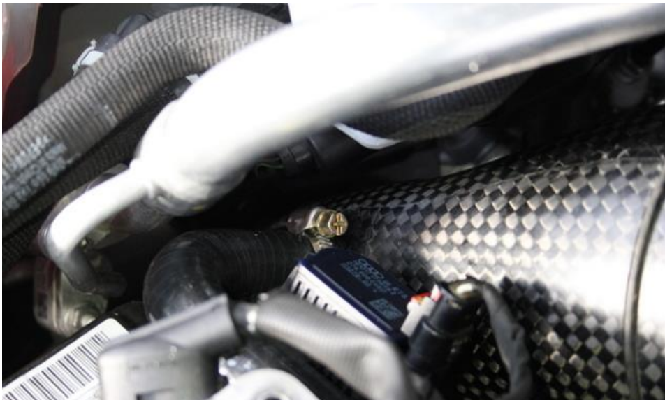
27. Now tighten the small clamp around the breather silicon at the carbon tube end. Again – do not over tighten.
