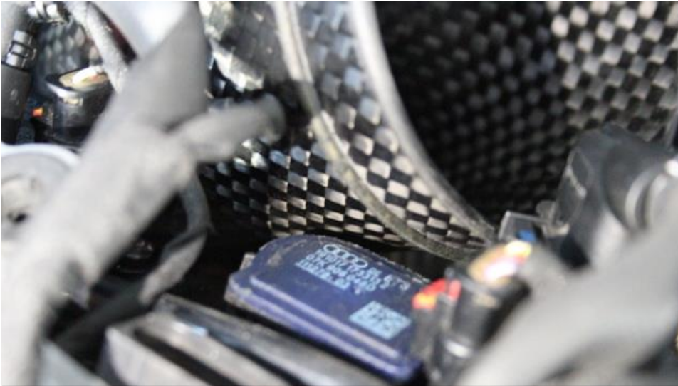
25. The Carbon tube should be almost touching the first sensor block.
