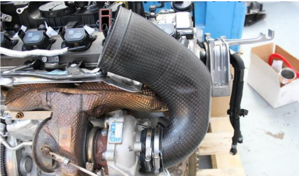
19. Push the inlet tube firmly into the silicon and ensure it is fully in. Do not tighten the clamp yet.
