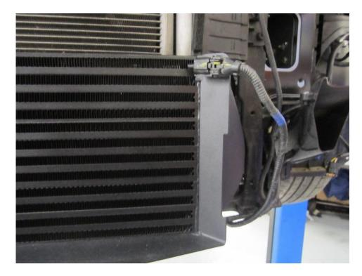
**18**. The Forge hard pipe and silicone hoses can now be installed, first fit them together loosely as shown in the picture off the car. Slide the hose onto the intercooler then attach the 90-bend hose to the OE pipe, with both pipes attached move the hard pipe until the bracket lines up with the fastener hole and re-fit the fastener in place. Finally tighten up all the hose clamps with a 7mm rachet or flat blade screw driver.
