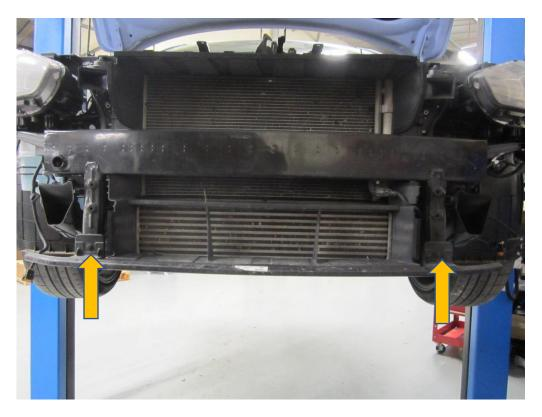
8. Unplug and remove the temperature sensor from the crash bar. To remove the sensor, use a trim removal tool or flat blade screw driver to lever the sensor away from the crash bar.
