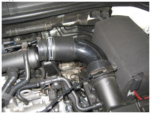
2. Remove the small 8mm bore pipe form the side of the airbox
