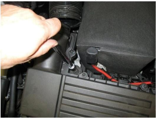
4. Working on the front edge of the airbox, push the clips in on the side of the cold air feed to work it loose, then unclip the water hose from the rear of the feed, and lift the feed clear of the airbox.
