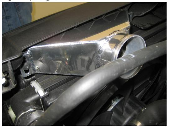
8. Fit one of the Forge 76-70mm reducers to the stock intake pipework, followed by the 90 degree aluminium bend, and the straight 76mm joiner. Use 60-80mm jubilee clips on the 70mm pipe, and 70-90mm on the 76mm pipe. Connect the small bore 8mm pipe to the barb on the aluminium bend.
