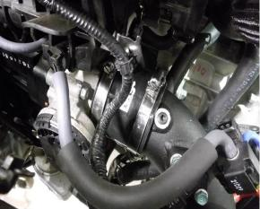
13. Mount the solenoid to the FMBP7 hard pipe using the m6 fastener removed earlier. Use the vacuum hose supplied with the kit to replace the original hose as this will be too short to reuse. This needs to be used for the diverter valve vac hose also, Cut the vacuum hose to the required length with the use of side cutters then use the provided small cable ties to secure the vacuum lines in place.
