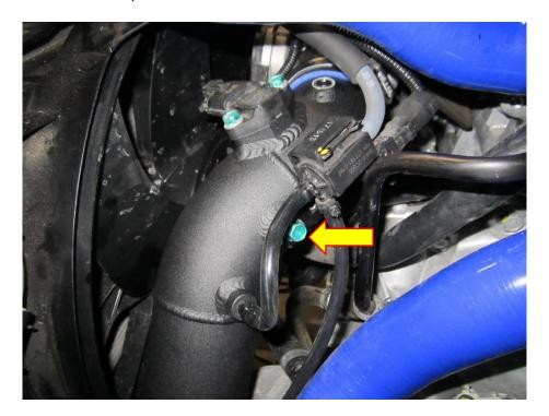
14. Re-fit the diverter valve and connect the vacuum hose, use the large cable tie to secure this vacuum hose to the lower radiator hose. Do not over tighten this as it can pinch the vacuum line. Using a 7mm sockt and ratchet tighten up all the hose clamps.
