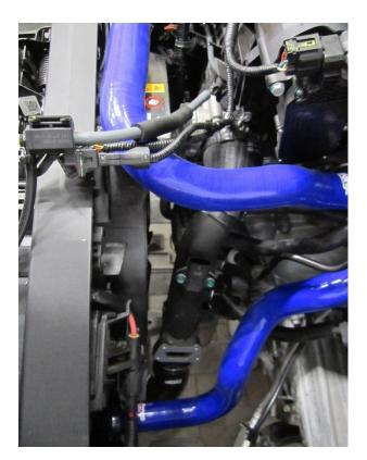
9. Using an 8mm socket and ratchet release both hose clamps attaching the boost pipe to the vehicle, there is one which holds the rubber joiner hose to the throttle body and one which holds the 90 degrees joiner hose to the intercooler. Some clamps may have a cover over the worm drive, this can be removed with plyers.
