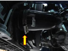
10. With the boost pipe out of the vehicle, use a 10mm socket and ratchet to remove the X 2 M6 fasteners attaching the map sensor to the boost pipe.
