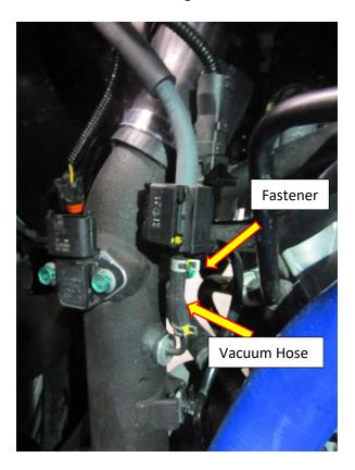
8. Move the solenoid and map sensor loom out of the way to make the removal of the boost pipe easier.
