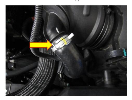
4. Using plyers loosen both spring clamps to allow the removal of both breather hoses at the other end of the inlet pipe. Using a 10mm socket and ratchet loosen the hose clamp attaching the inlet pipe and joiner to the turbo elbow, you will now be able to remove the air box and intake pipe together as one part.
