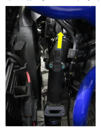
7. Using long nose plyers loosen the sprung hose clamps securing the small vacuum hose from the solenoid to the boost pipe and remove the pipe completely. Using a 10mm socket and ratchet remove the M6 fastener holding the solenoid to the OE boost pipe.
