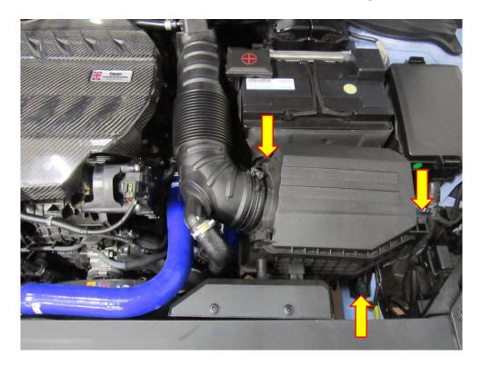
2. Using a flat blade screwdriver/ trim removal tool push the pin in the centre of the fastener inwards, then prise up the fastener to remove it.
