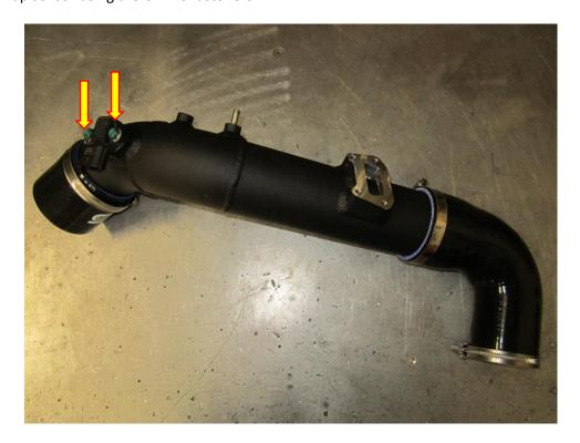
12. Fit the FMBP4 into place in the vehicle's engine bay, as shown in the picture below.
