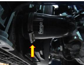
10. With the boost pipe out of the vehicle, you now must remove the map sensor which attached to the boost pipe with two m6 fasteners. Use a 10mm socket and rachet/spanner to remove them.
