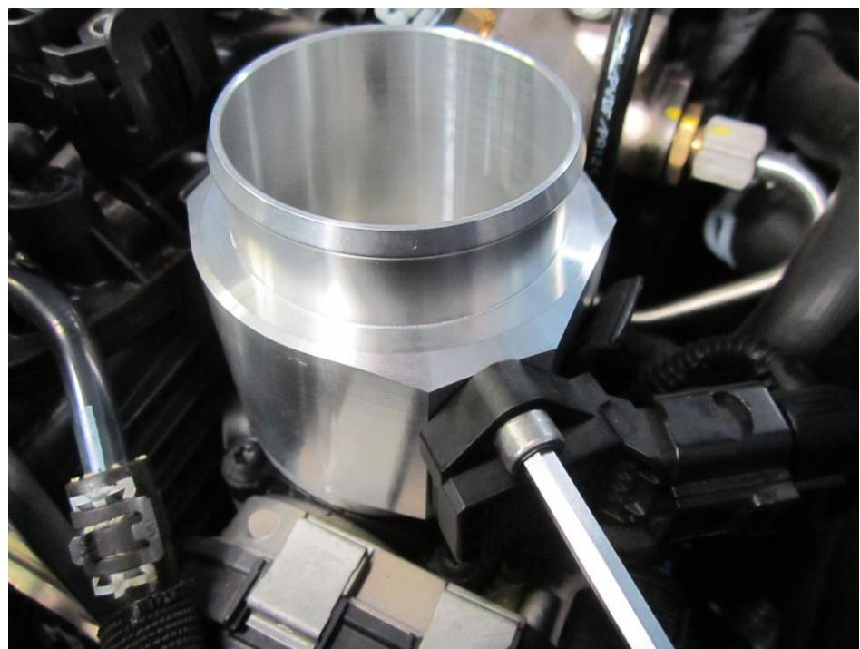
12. Fit the large silicon boost pipe into position and tighten the hose clamps with your hose clamp driver. Tighten the hose clamp at the small end first as this ensures the boost pipe is sat in the correct position .
