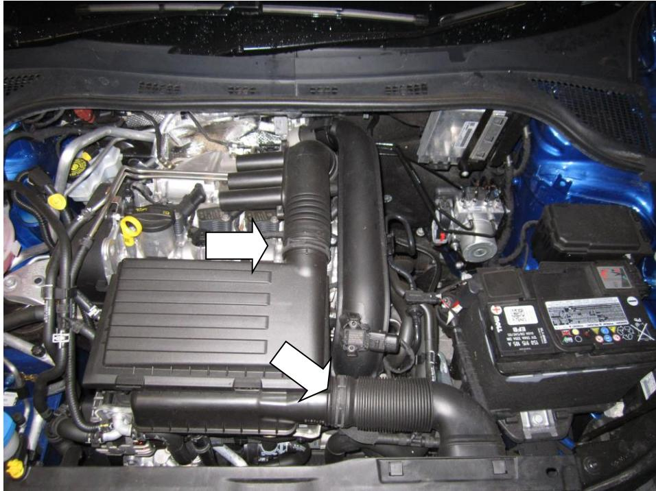
2. Now remove the inlet hose from the slam panel by pushing down on the retaining clips as pictured below.
