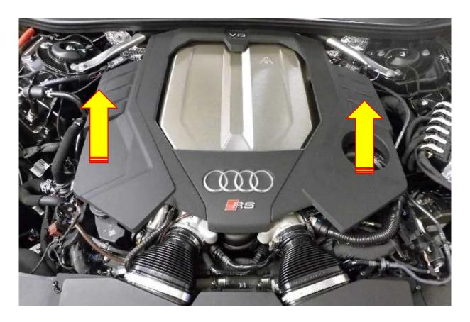
2. Using a T25 torx drive remove the 7 fasteners that hold the airbox lid in position. Please note these do not come fully away from the airbox lid.
