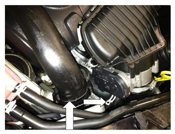
2. Remove the noise generator pump by simply pulling towards you.
