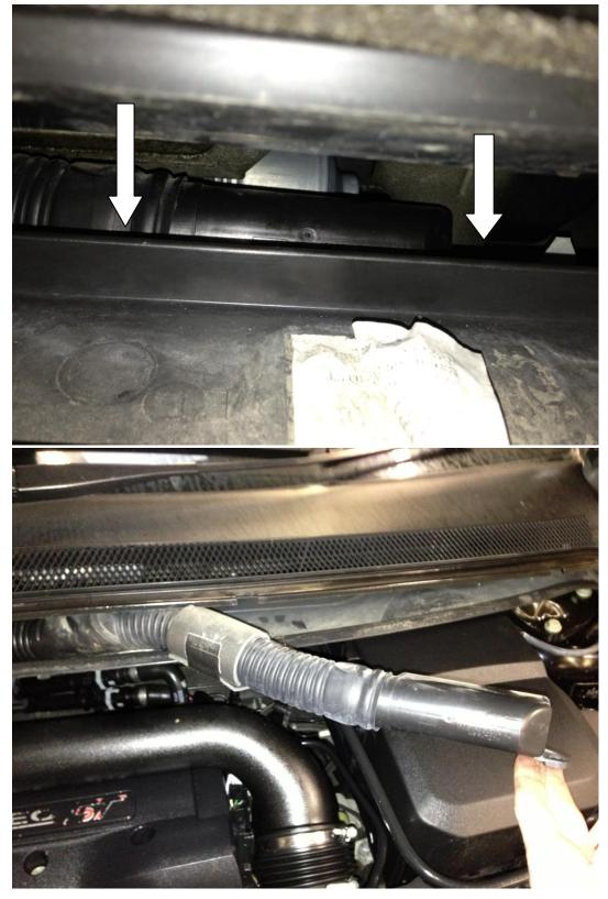
6. Using a T30 Torx driver, remove the two T30 torx bolts holding the cam cover to the engine.
