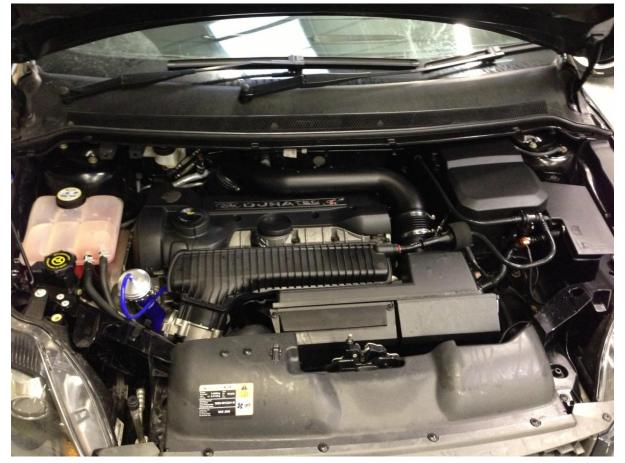
Tools Required: Hose clamp driver T30 Torx Hose clamp removal tool or pliers 10mm spanner Phillips screw driver  Firstly, remove the top noise generator pipe from the pump by pulling upwards. Then using a hose clamp removal tool, remove the hose clamp and pipe shown by the arrow below.
