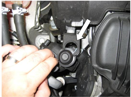
3. Using a 10mm spanner, remove the two 10mm bolts holding the bracket to the engine. The bracket is no longer used.
