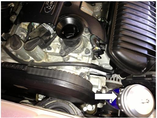
9. With the cambelt cover removed you will now see the small black vacuum pipe running along the top of the engine. Cut this pipe in the area shown in the picture below. Once cut simply place the plastic "T" piece provided into the hose.
