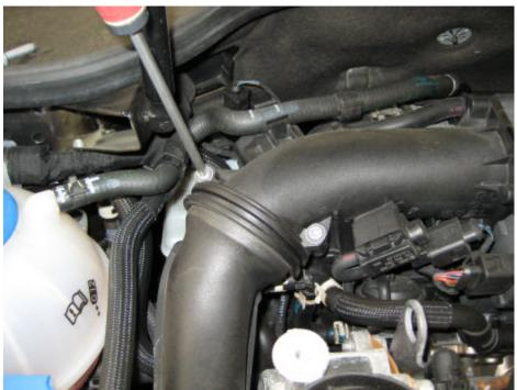
6. Pull the intake hose away from the turbo. This will require a fair amount of force as the hose is held in place with a rubber o-ring.
