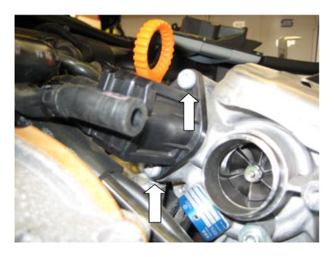
8. Remove the valve from the side the of the turbo, and make sure the o ring is in good condition. If not, replace it with a new one from your nearest Volkswagen dealer. Insert the valve into the Forge dump valve adapter, and place it back in the side of the turbo. Access is pretty tight so you may need to move the hoses underneath the valve around.
