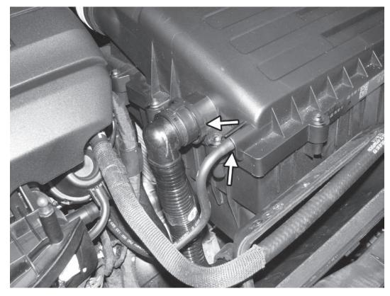
1) Remove the vacuum line from the front right corner of the factory airbox by pulling it off. Then, if equipped, remove the connection to the secondary air pipe by pressing down on both sides of the fitting and pulling away from the airbox.
