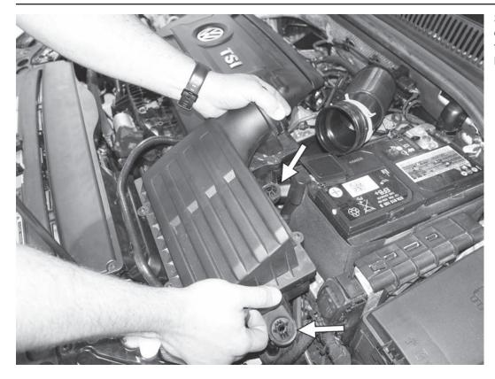
3) Firmly lift up on the back and side of the factory airbox, separating it from the two rubber mounts on the left and back sides of the airbox.
