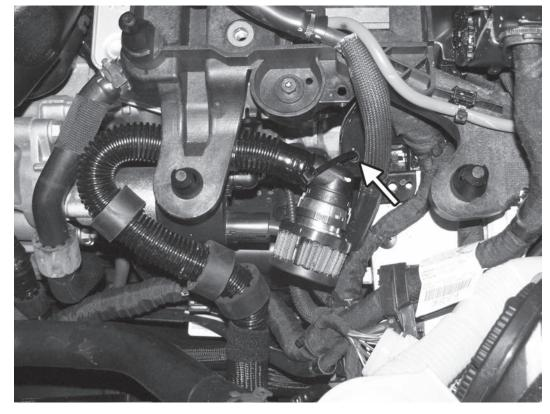
7) Snap the secondary air filter to the factory fitting on the secondary air pipe. Bend the pipe down to tuck it out of the way and secure it with a cable tie.
