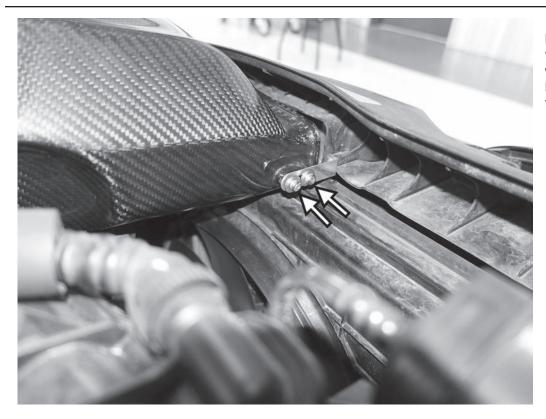
17) Using the supplied blue thread locker on the screws, install and tighten the two 3mm allen screws with washers to hold the front "L" bracket to the mounting boses on the front right of the APR intake.
