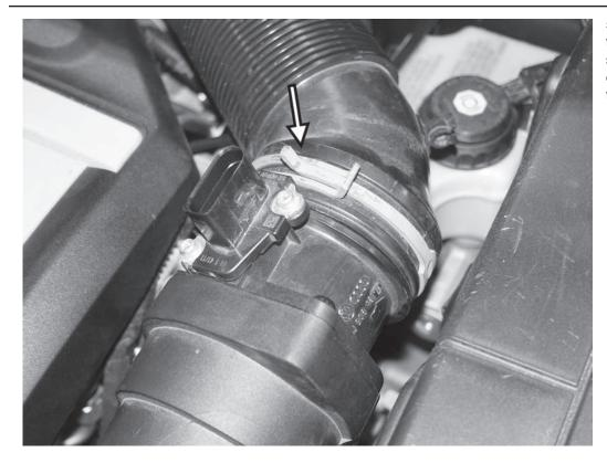
5) Squeeze the hose clamp holding the accordian inlet elbow to the back side of the MAF sensor, and slide the clamp off the MAF sensor. Separate the inlet elbow from the MAF sensor.
