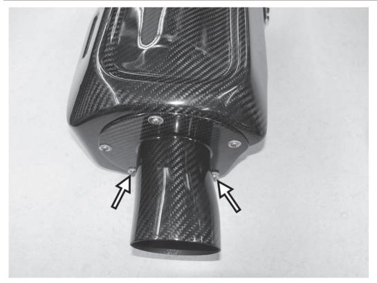
11) On the APR intake, remove the two lower, rear 3mm allen screws from the filter access panel on the back of the intake.
