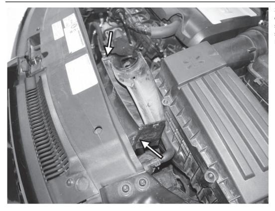
3) Press in the tabs on both sides of the inlet scoop, and rock the inlet scoop back to separate the inlet scoop from the radiator core support. Remove the inlet scoop from the car.
