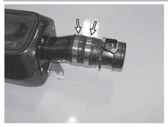
13) Using the supplied silicone coupler and two hose clamps, loosely install the MAF sensor to the back of the APR airbox in the same orientation as the with the stock sensor.
