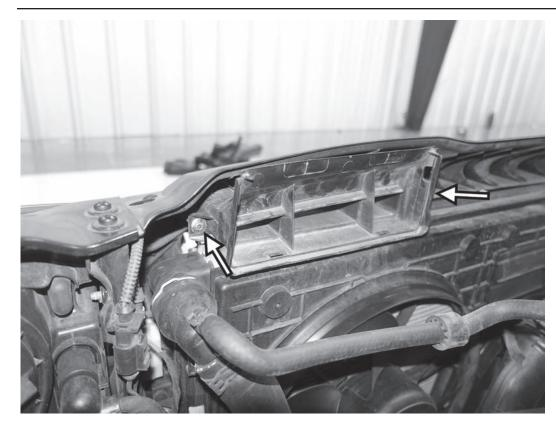
9) Unscrew the two T25 screws holding the front of the airbox inlet scoop from the back of the radiator core support.
