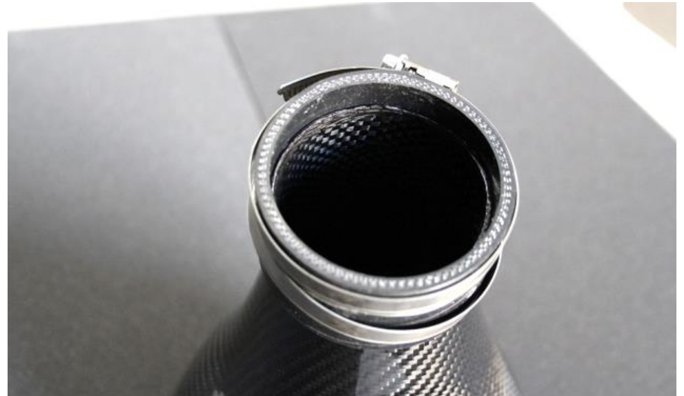
20. Push the silicon onto the housing so that only around 10mm is showing from the inside. This will give you more clearance when installing the housing.
