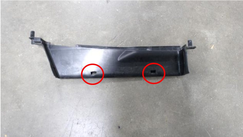
29. Take the front duct trim from step 5 – we will secure the carbon scoop to the circled holes.
