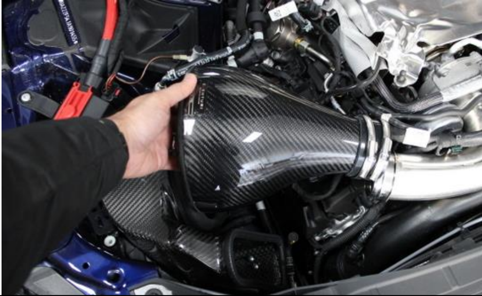
21. Lower the housing between the duct and the turbo inlet tube. The Eventuri Plaque should face upwards.
