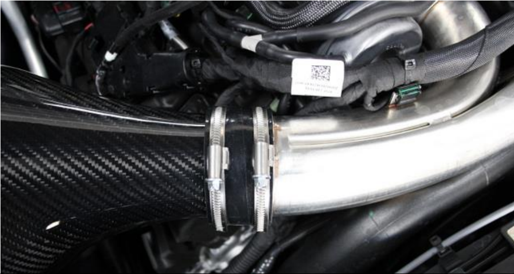
25. Pull the silicon coupler over the turbo inlet tube but don't secure the hose clamps yet.
