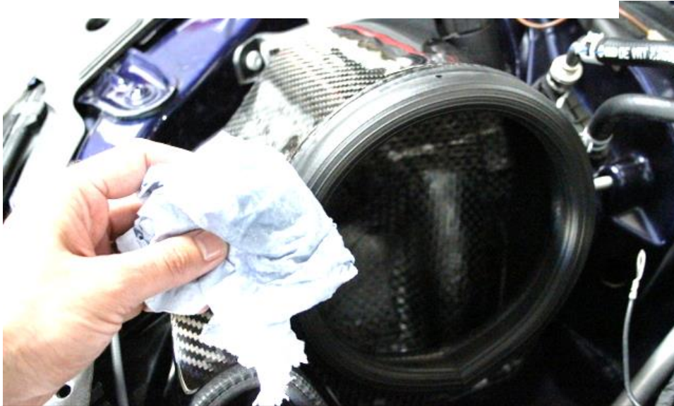
17. Spray some lubricant onto a cloth and wipe the front of the rubber seal around the duct so that the housing can be easily pushed into place without pulling the rubber seal out.
