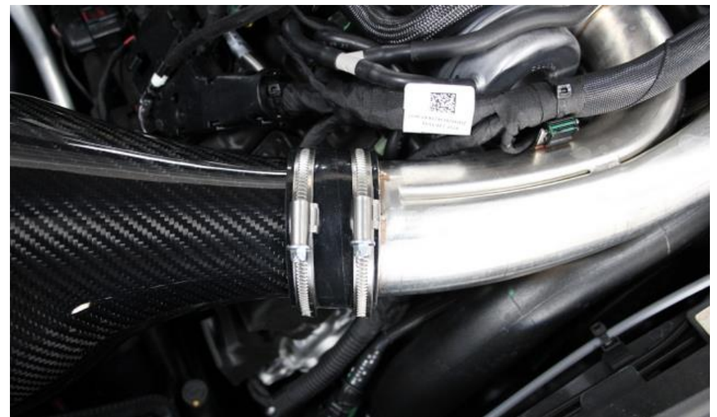
28. Now secure the hose clamps. Do not over tighten.
