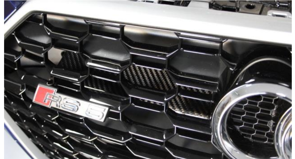
30. The scoop should sit behind the front grill as shown.
