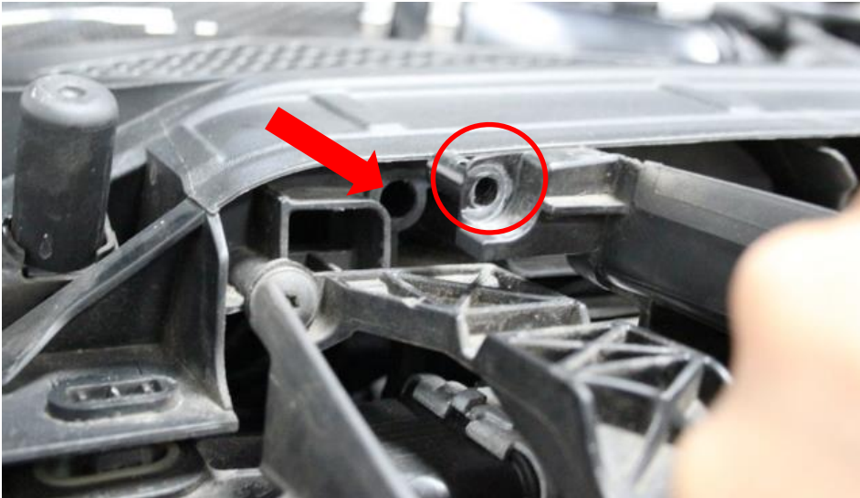
29. Relocate the front duct trim into its original position – the boss for the torx screw should go into the hole in the slam panel on both sides.
