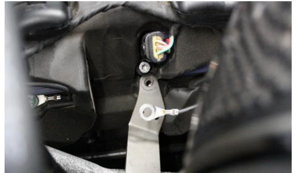
24. Rotate the housing so the bracket lines up with the threaded hole on the engine which had the Torx Screw removed in step 14.
