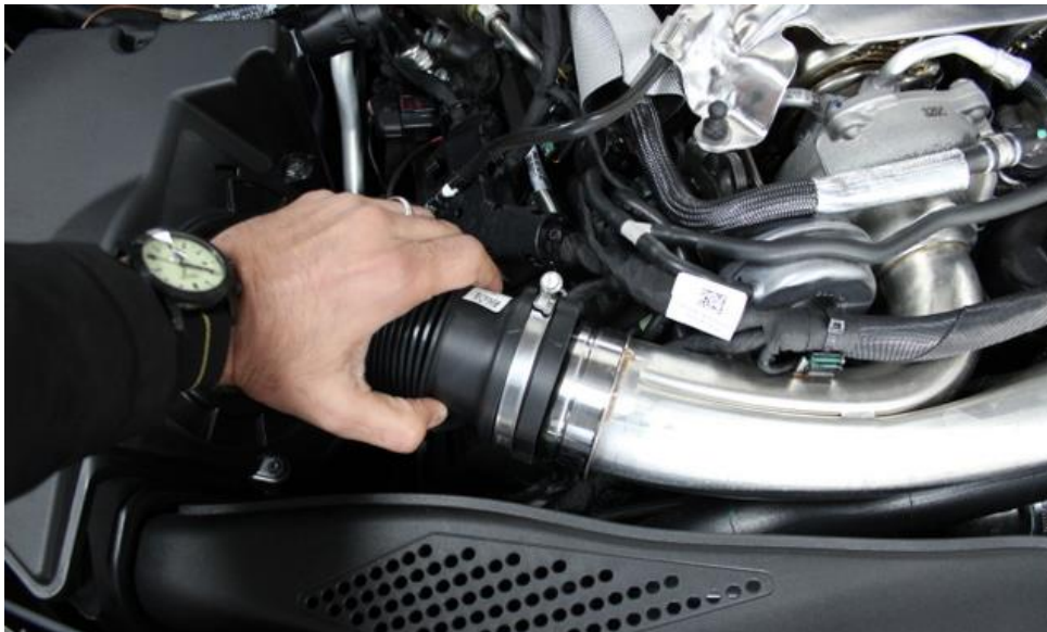
7. Loosen hose clamp connecting the flexible tube to the turbo inlet tube and pull it away.
