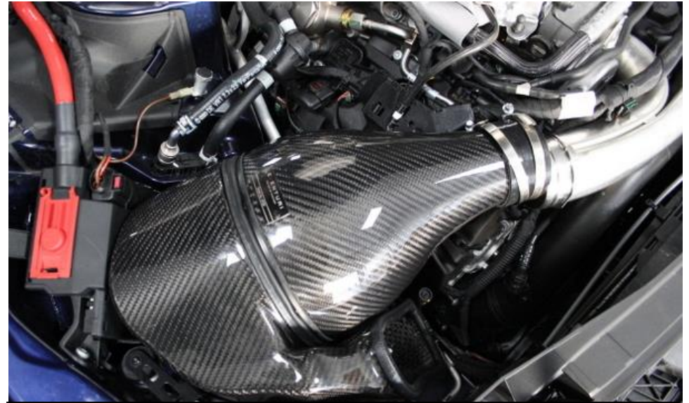
22. Push the Housing down so that the front lines up with the rubber seal on the duct. While aligning it make sure the bracket lines up with the mounting hole – see next step.
