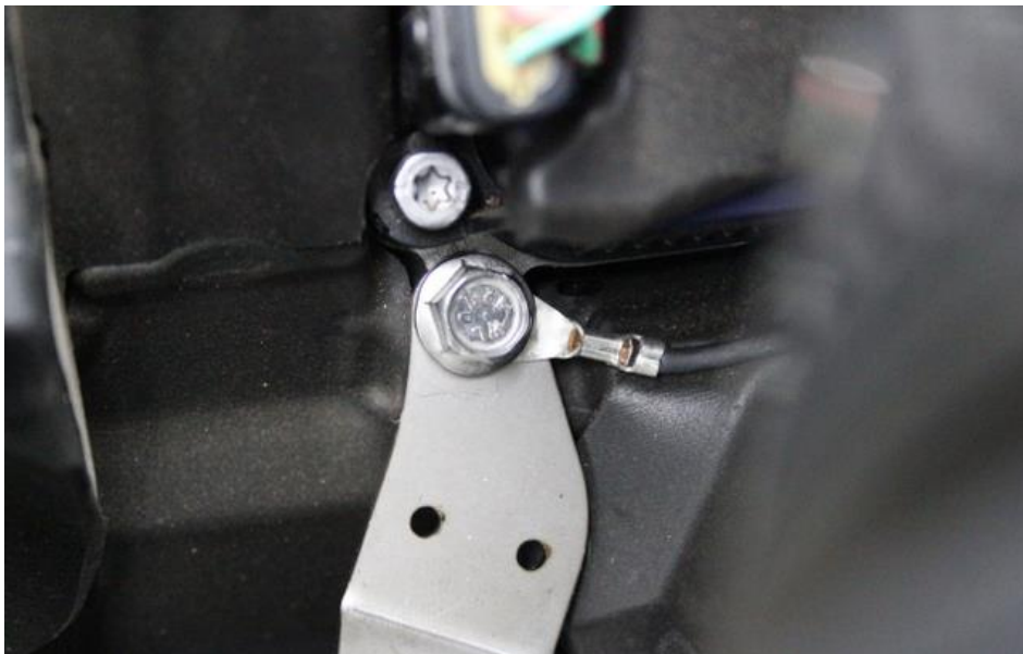
27. Secure the bracket using the supplied bolt – make sure the earth wire is also re-positioned and secured.
