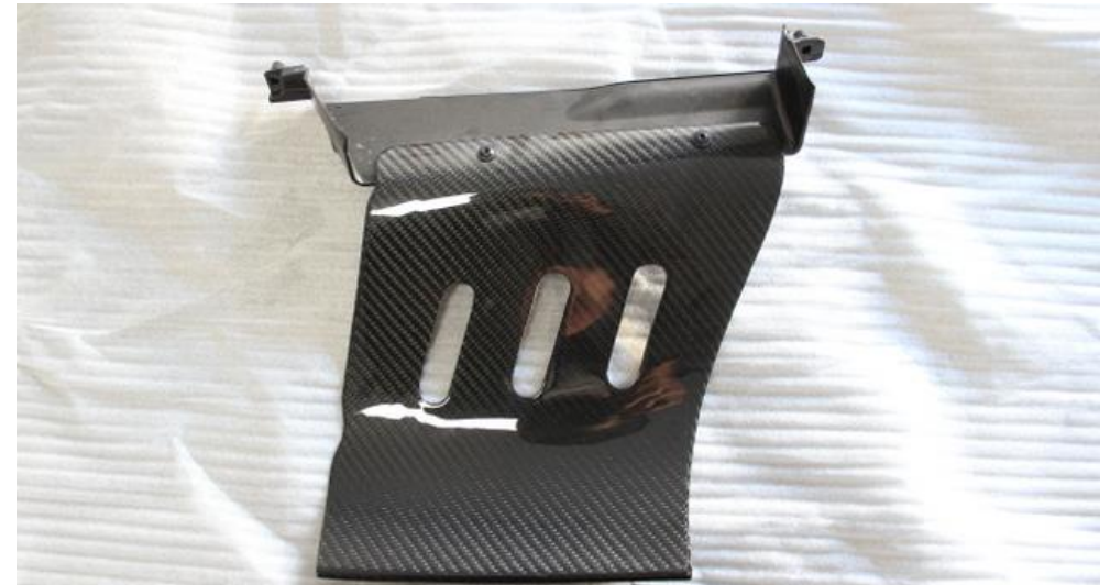
30. Locate the scoop as shown – secure with the supplied M5 black flange bolts and lock nuts – see next step.
