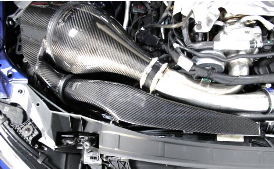
31. Push the carbon secondary duct into the main duct.
