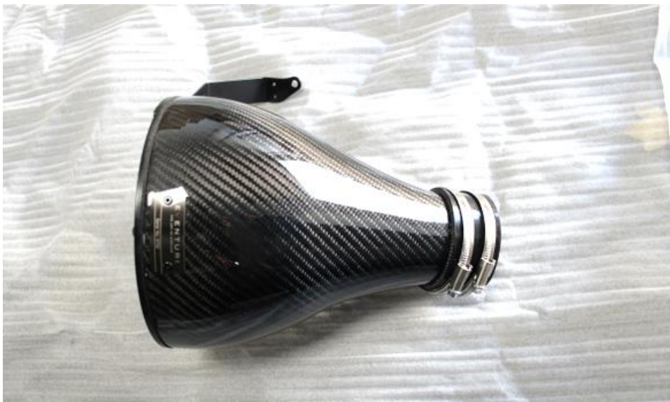
19. Push the Silicon coupler onto the housing and loosely place the hose clamps over the coupler.
