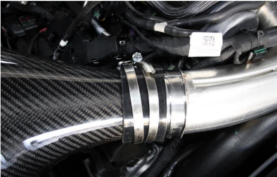
23. Line up the silicon coupler over the turbo inlet tube. While aligning it make sure the bracket lines up with the mounting hole – see next step.
